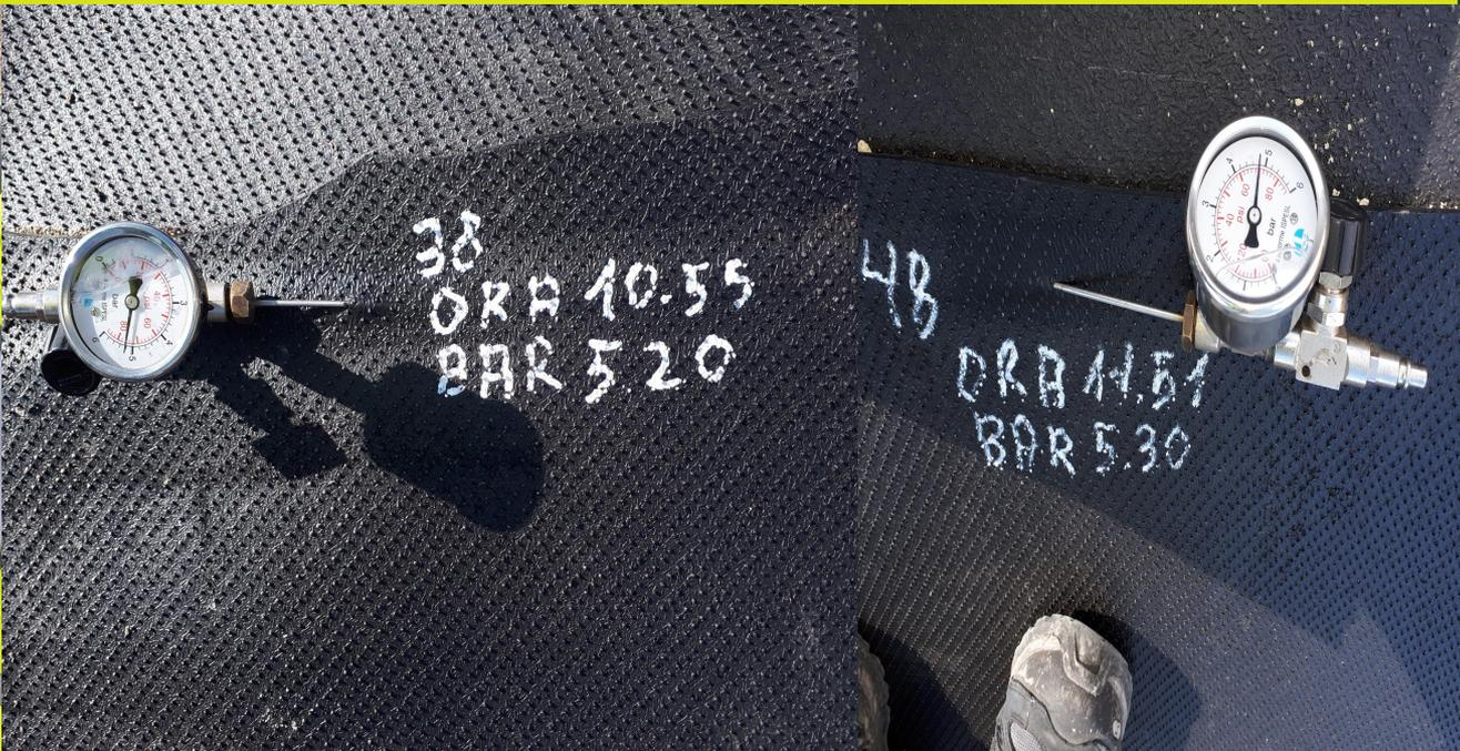
**-CONTROLLO SALDATURE DOPPIA PISTA CON CONTROLLO PNEUMATICO A STRAPPO**
